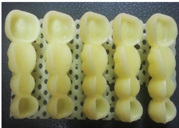
Fig. 4. Polymer temporary bridges, produced by stereolithography.
