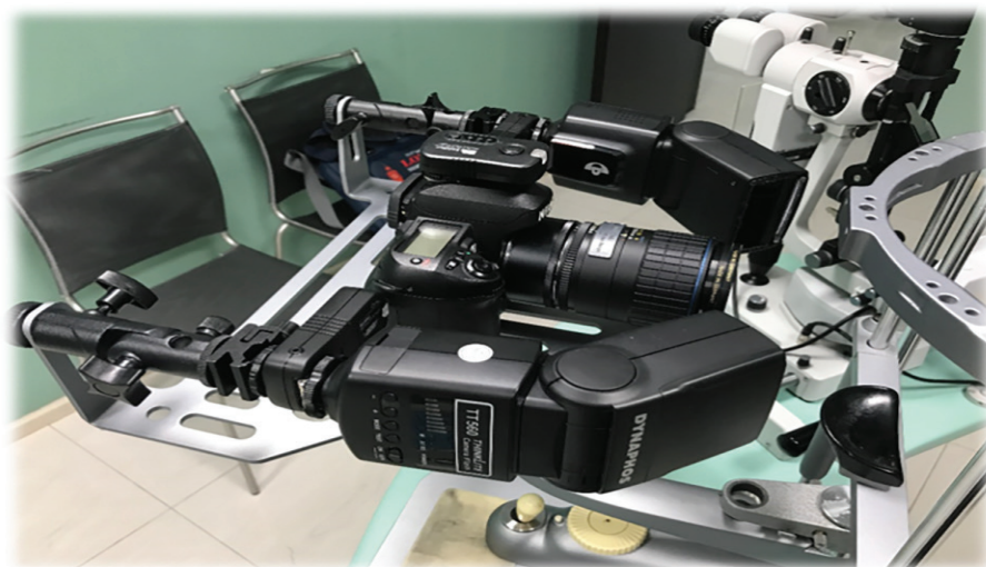
Fig. 2. Camera used for detecting ultraviolet autofluorescence in the study
