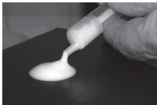
Fig. 4. Foam with high viscosity and stability
