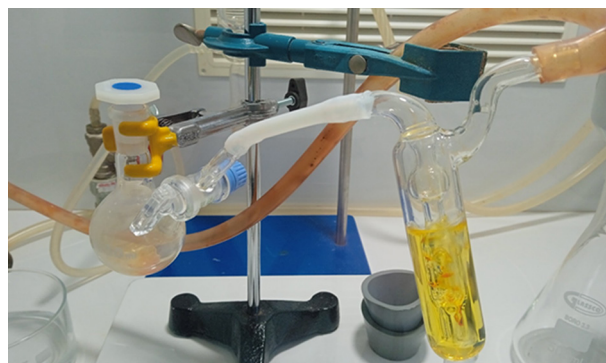
Fig. 4. A photograph of the experimental setup used for the production of bromine. In the same photograph, reaction equation 1 is also presented.
